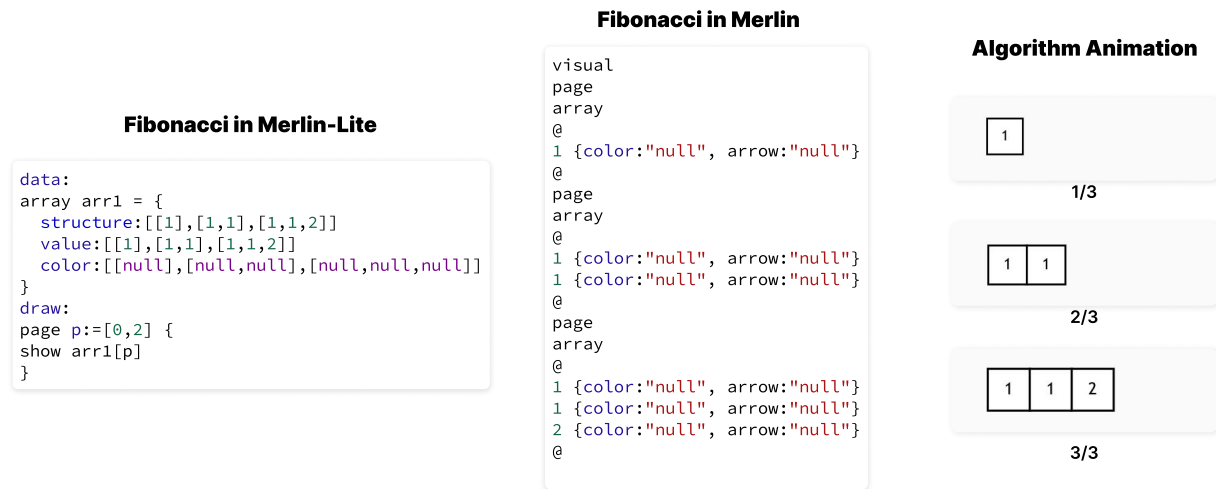
Figure 4: The different descriptions of Fibonacci array by MERLIN(right) and MERLIN-LITE(left)
